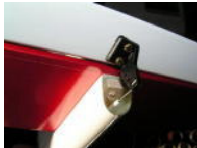
Elevator cable installed
