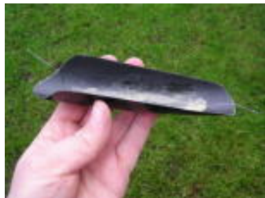
Canopy with epoxied-in wire
